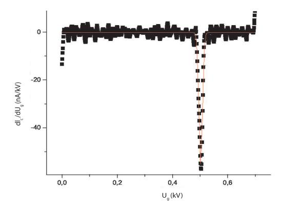
Figure 7:  $dI_c/dU_g$  vs.  $U_g$ . Points from fig. 6a. Drawn curve: Fit to  $f(x) = A \cdot exp(-(x - xc)^2/(2\sigma^2)), x = 10^3 U_g$ .  $xc = (502.26 \pm 0.09)$  V,  $\sigma = (6.39 \pm 0.09)$  V.
