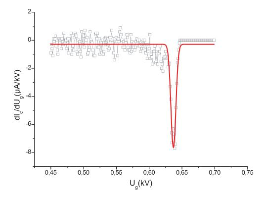
Figure 4: Differentiated proton cup current  $dI_c/dU_g$  vs.  $U_g$ . Points from fig. 3. Drawn curve: Fit to  $f(x) = A \cdot exp(-(x - xc)^2/(2\sigma^2)), x = 10^3 U_g, \sigma = (3.83 \pm 0.17)$  V.
