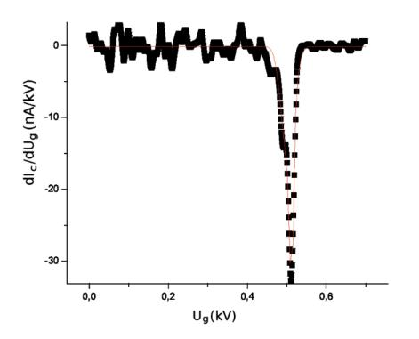
Figure 8:  $dI_c/dU_g$  vs.  $U_g$ . Points from fig. 6b. Drawn curve: Fit to  $f(x) = A1 \cdot exp(-(x - xc1)^2/(2\sigma_1^2)) + A2 \cdot exp(-(x - xc2)^2/(2\sigma_2^2)), x = 10^3 U_g$ . xc1 = 502.26 V,  $\sigma_1 = (16.07 \pm 0.41)$  V,  $xc2 = (512.03 \pm 0.19)$  V,  $\sigma_2 = (5.04 \pm 0.19)$  V.
