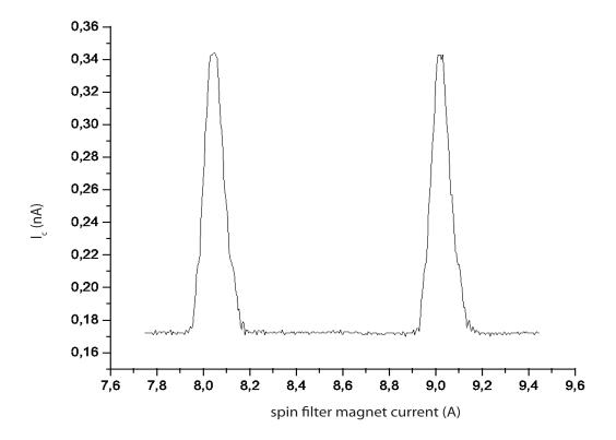
Figure 2: Cup  $H^-$  current  $I_c$  vs. spin filter magnet current. At the peak setting H(2s) and H(1s) atoms appear behind the filter, whereas at the valley setting (between the peaks) only H(1s) remain.
