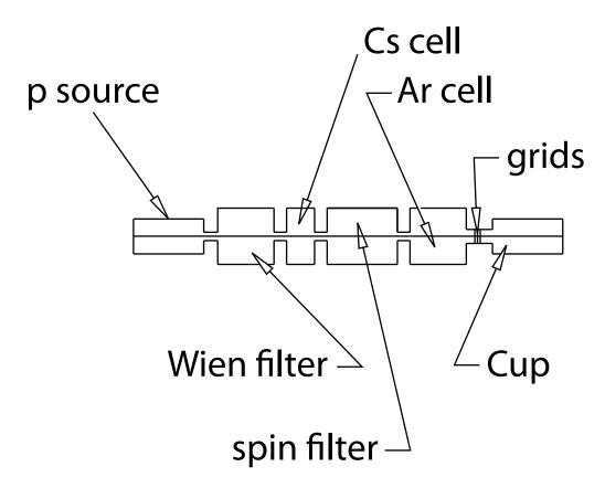
Figure 1: Sketch of the mockup setup to measure the kinetic energy difference of  $H^-$  ions produced by charge exchanged H(2s) and H(1s) atoms within an Ar cell.
