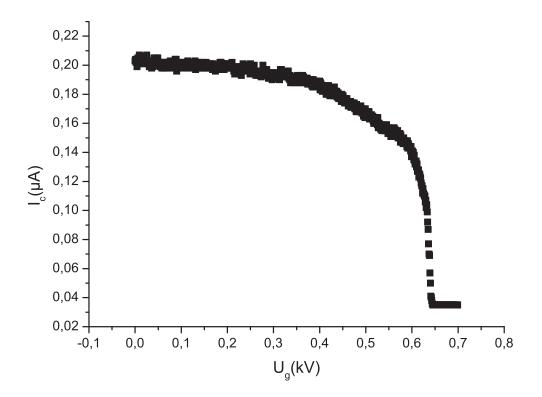
Figure 3: Proton cup current  $I_c$  vs. counter field grid voltage  $U_g$ . The plasma source accelerating voltage was set to about 640 V.
