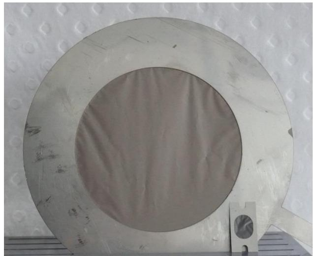
Figure 1: 80mm ultra-thin carbon foil for the ASACUSA experiment at CERN. On the bottom right a standard 90mm<sup>2</sup> frame as used at the MLL experiments is shown.
